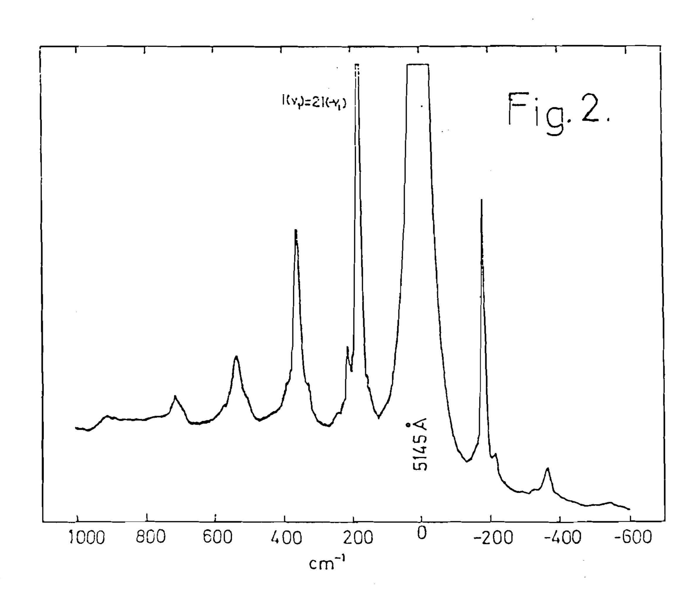
The Raman spectra were taken with a JOBIN YVON Ramanor HG-2S Spectrometer and a Spectra Physics Model 165-03 Ar ion laser. The required power of the laser was 20mW.
