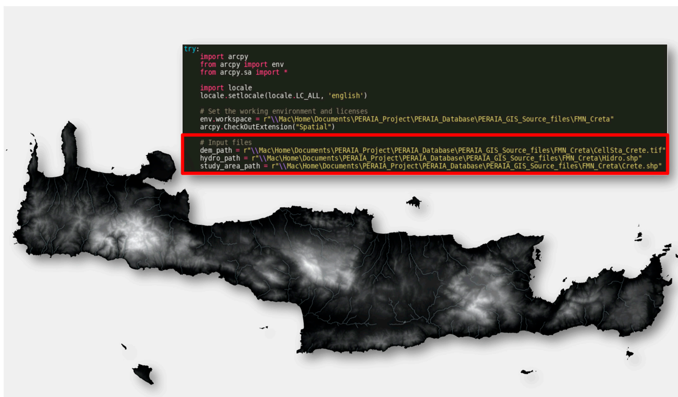
Figure 7. (Above) Setup of the working environment through code. (Below) Digital Elevation Model (25 m resolution) of the island of Crete, overlaid with the hydrographic network. Areas of highest flow accumulation, as identified in this study, are highlighted.
