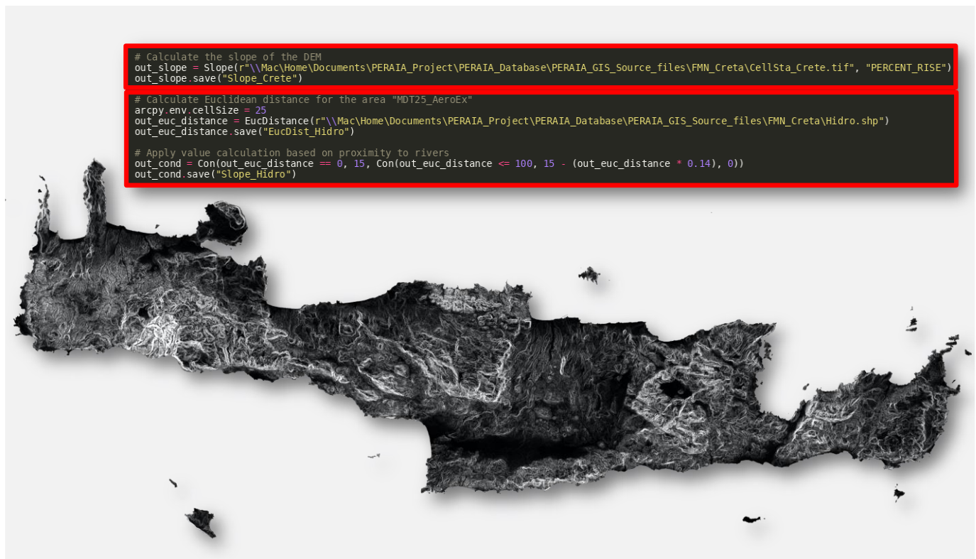
Figure 8. Procedure for calculating slope (expressed as a percentage) and assigning a graduated cost to areas intersecting the hydrographic network.
