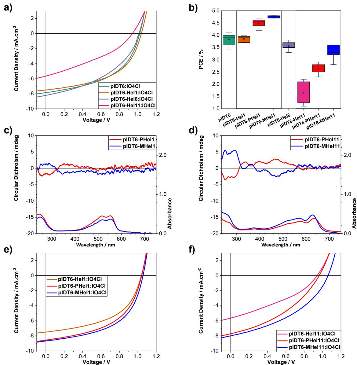
**Figure 4.** (a)  $J-V$  curves of the cells based on racemic polymers, (b) box plot of the PCE of all the solar cells studied. (c, d) ECD (top) and UV-Vis absorption spectra (bottom) of the thin-film blends of pIDT6-(P/M)Hel1:IO4Cl (c) and pIDT6-(P/M)Hel11:IO4Cl (d). (e, f)  $J-V$  curves of the cells based on racemic and enantiopure polymers on 1% helicene loading (e) and on 11% helicene loading (f).
