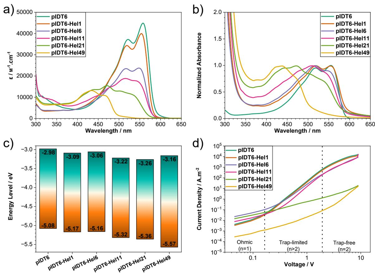
**Figure 2.** a) Experimental absorption spectra of **pIDT6-Hel(x)** polymers in CHCl<sub>3</sub> solutions ( $c = 10^{-5}$  M) at room temperature; b) Experimental normalized absorption spectra in solid-state spin-coated films of **pIDT6-Hel(x)** polymers at r.t.; c) Energy levels of the racemic **pIDT6-Hel(x)** polymers stemming from APS and ss-UV-Vis; d) Hole mobilities of the racemic **pIDT6-Hel(x)** polymers from SCLC measurements.
