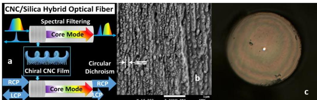
**Figure 1** a) Schematic diagram of the principle of the CNC integration on the facets of optical fibers. RCP and LCP (Right and Left Circular Polarization) b) SEM image of the cross-section of the layered periodic CNC film. c) Optical microscope image of a fiber facet with CNC film.
