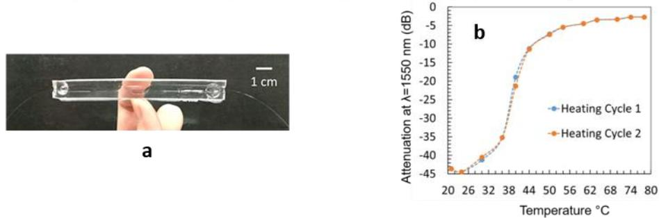
**Figure 2** a) Photograph of the PDMS-embedded tapered fiber device. b) Optical attenuation of a thermally tuned tapered microfiber embedded in PDMS polymer Heating Cycle 1 (heating), Heating cycle 2 (cooling).
