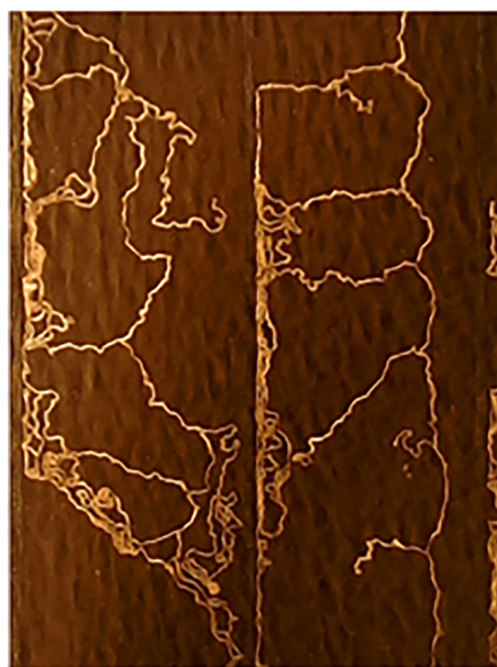
FIGURE 9 A close-up image of worm like defects in two interconnected cells of a CIGS module exposed to partial shading stress. Reprinted with permission of Bakker et al. 104
