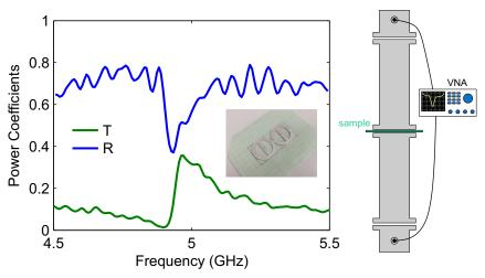
**Figure 5.** Measurement of the 3D-printed conductive unit cells within the WR-187 rectangular waveguide. The reflection ( $R = |S_{11}|^2$ ) and transmission ( $T = |S_{21}|^2$ ) power coefficients are plotted in the frequency range of 4.5–5.5 GHz.
