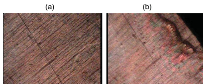
FIG. 8. (Color online) Optical microscopy observation of a piece of film (a) before and (b) after heating above the denaturing temperature of DNA.
